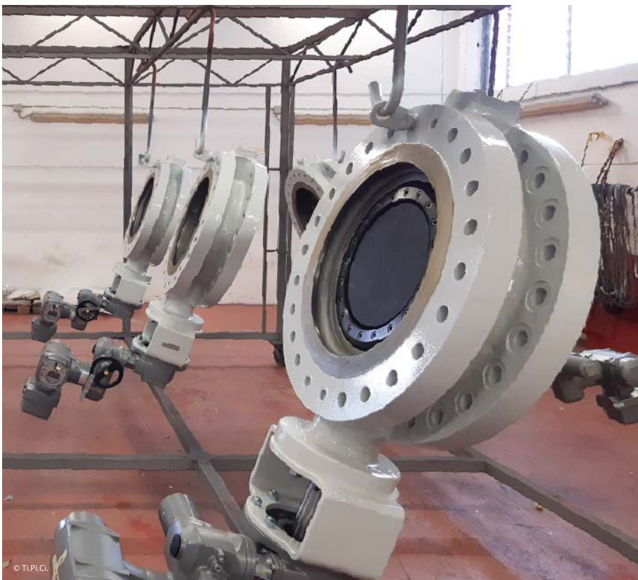
Some valves painted with the waterborne protective system developed by Ti.Pi.Ci.
