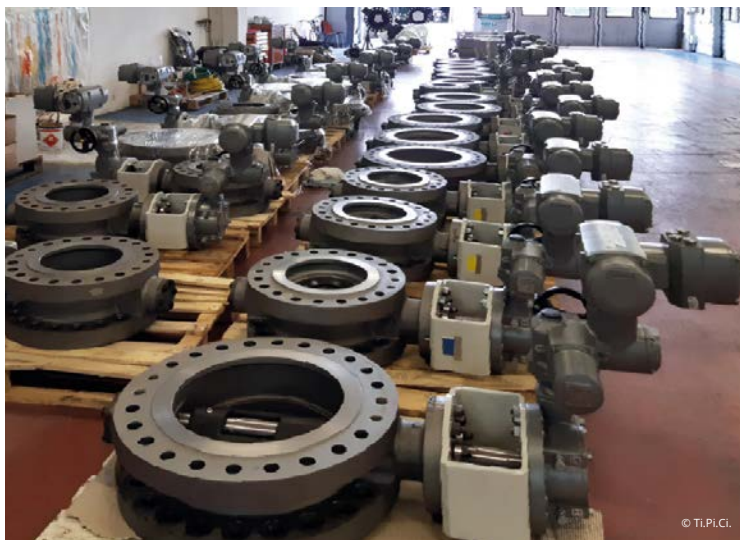
Valves awaiting surface treatment.
