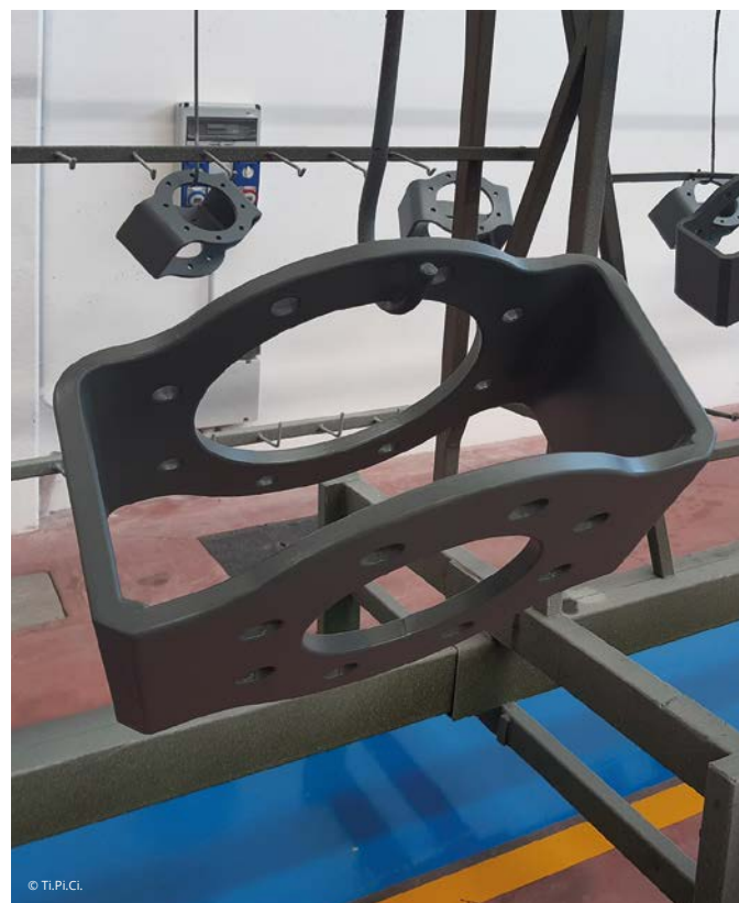
The detail of some brackets following the application of the first layer.
